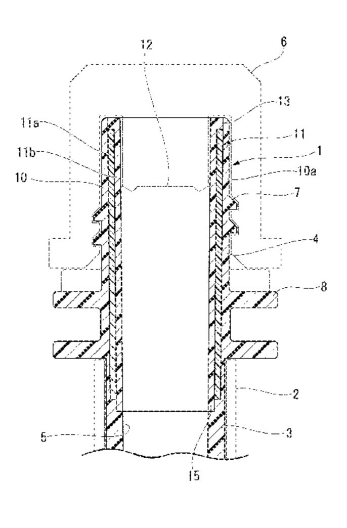
one end portion side in an axial direction of the covering layer (11b) and the outer peripheral surface of the covering layer (11b), which protrudes from an end portion in the axial direction of the blocking layer (11a) are embedded in the base resin in contact with the base resin.
