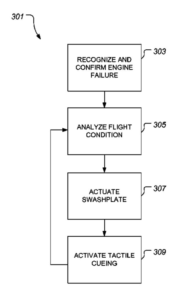
system can reduce workload by assisting the crew with controlling rotor speed and forward speed during stabilized autorotation.
