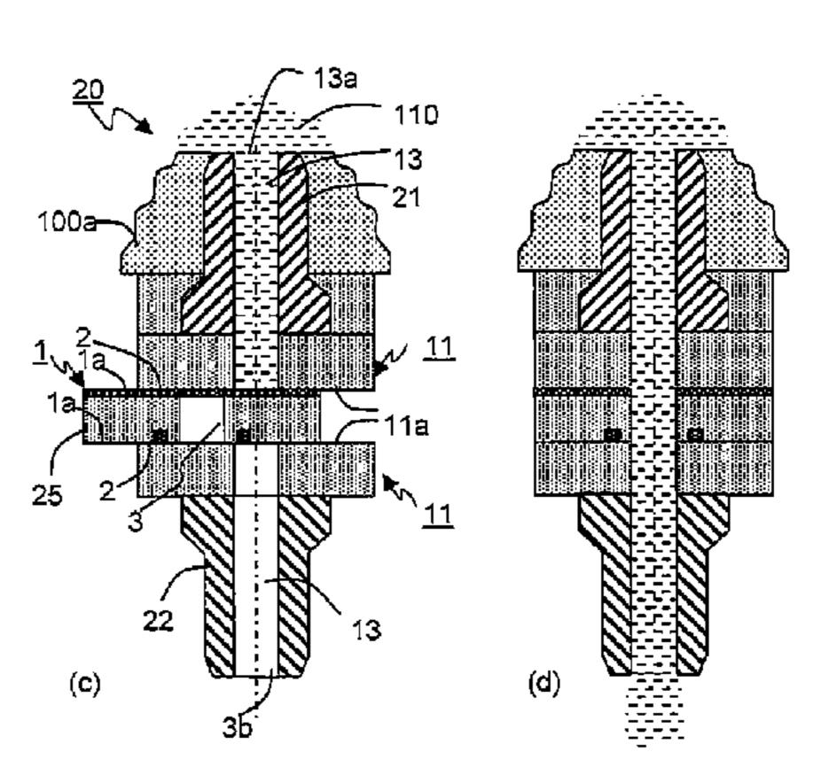
first and second coupling surfaces of the first and second elements. The sealing member comprises a thermally intumescent material.
