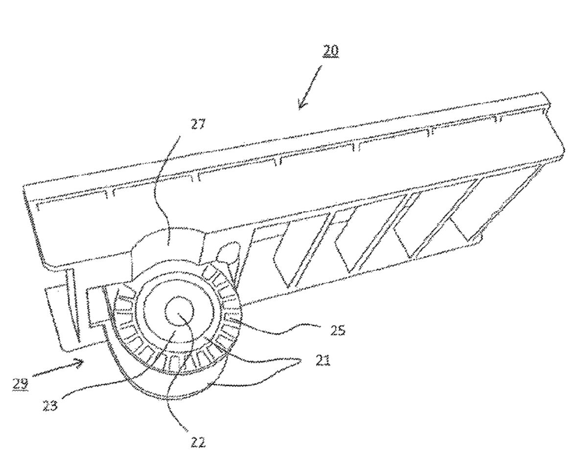
one third building element comprising a third type of hinge part which is complementarily configured in such a way that the hinge parts on the first and third elements can be interconnected, whereby both the second type and the third type of hinge parts are provided with a toothing.
