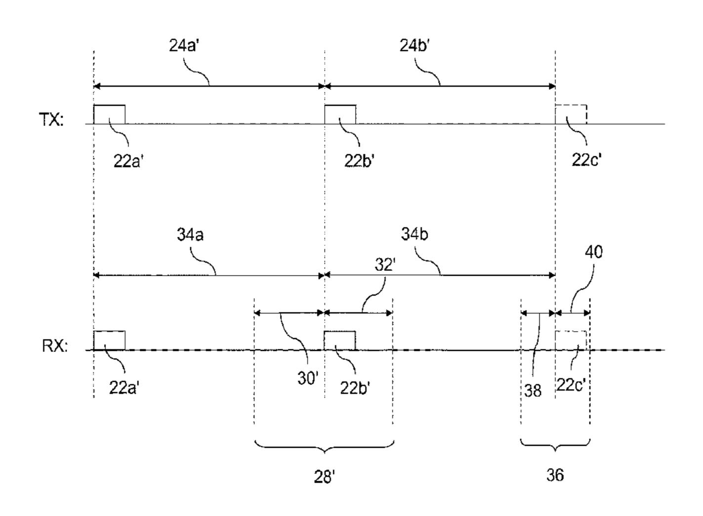
elapsed between the respective receipts of two of the connection-event data packets (22a', 22b') received by the receiver (12) minus a correction factor (38).
