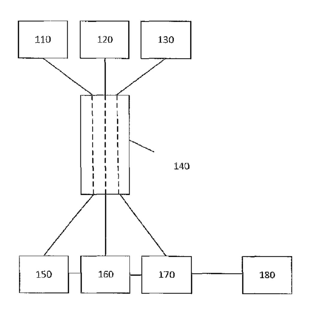
control signal is communicatively connected to a near end of a second secure communication tunnel through the nonsecure communication network. A far end of the first secure communication tunnel is communicatively connected to an activating input of a first barrier circuit, and a far end of the second secure communication tunnel is communicatively connected to an activating input of a second barrier circuit.
