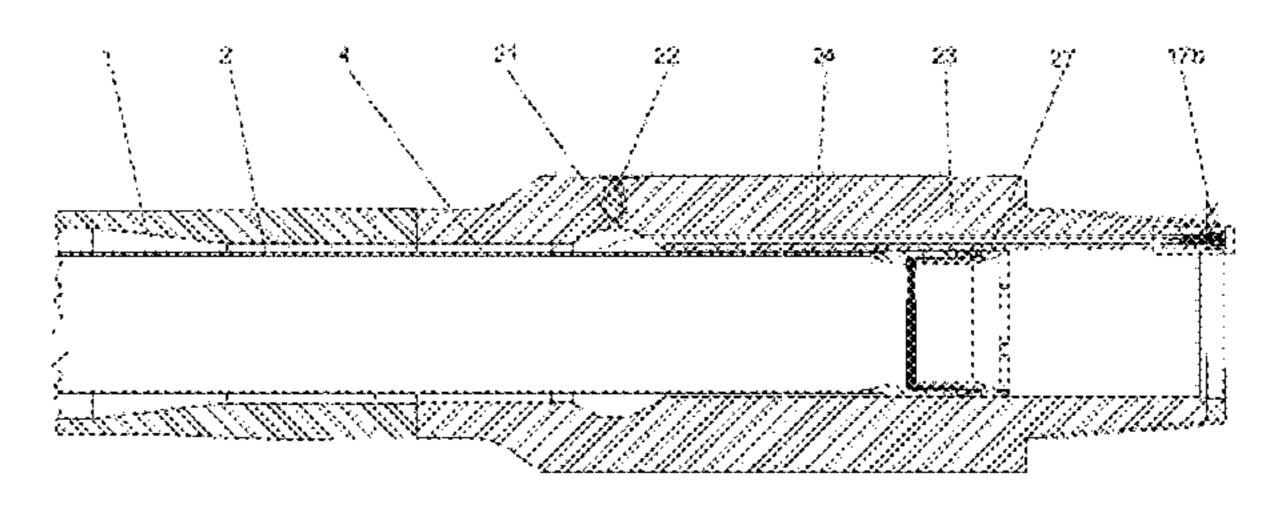
a hollow space (3). At least one electrical conductor (4, 7, 8, 9) is arranged on one outer side of the inner pipe.
