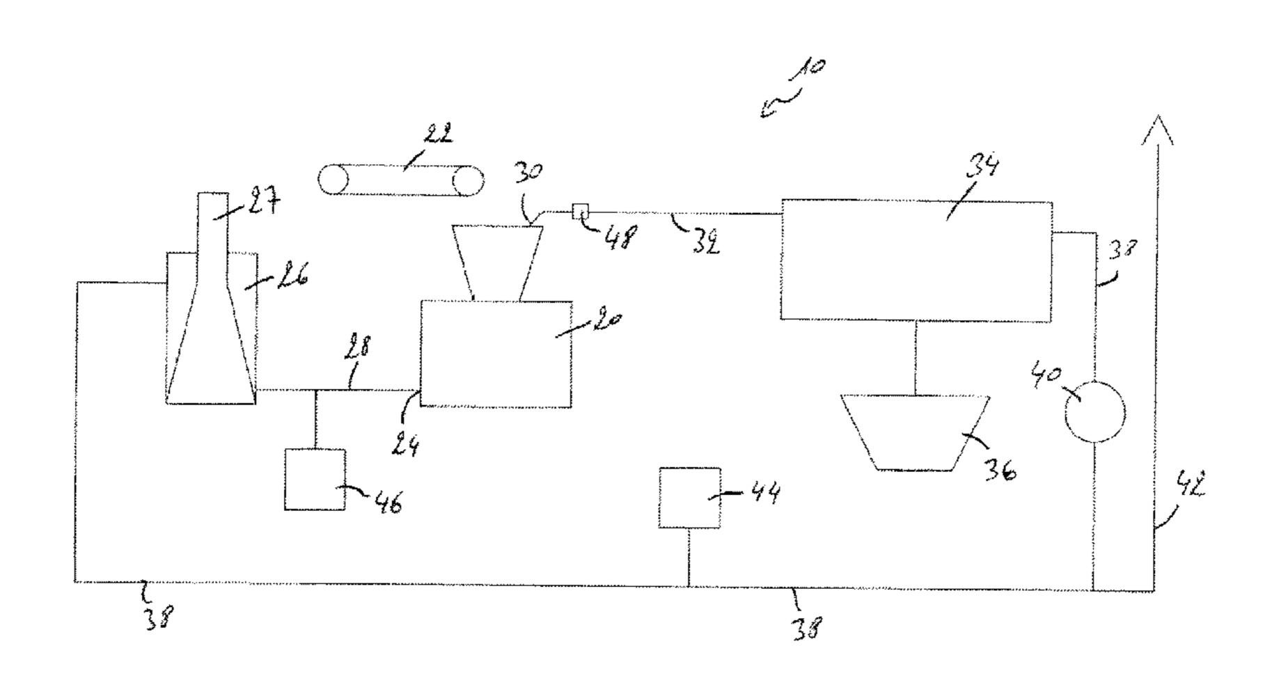
controlling a volume of water injected into the heated drying gas before feeding it into the pulverizer (20).
