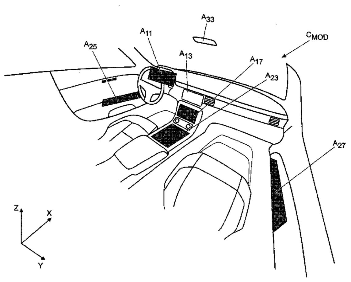
method comprises controlling an illumination source that is associated with the determined one of said plurality of areas of interest so as to highlight a visual zone associated with the vehicle.
