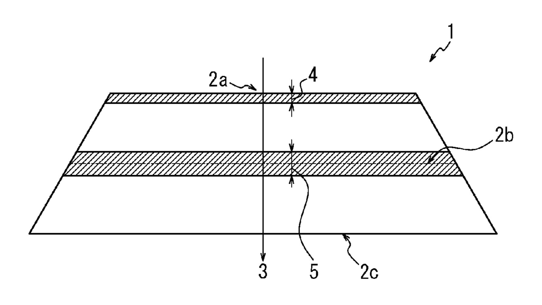
a median center between a tread portion outer surface and a bottom surface in the direction perpendicular to the tread surface.
