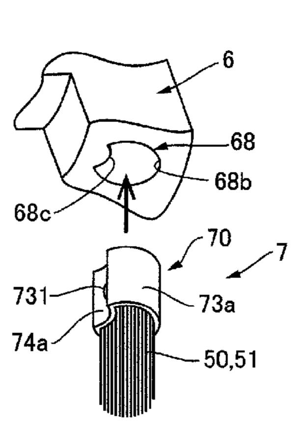
direction L. In a case where any of the linear member aggregates has a failure, such as breakage, only the failed linear member aggregate needs to be replaced. Thus, it is not necessary to discard the entire brush-like grinding stone. Consequently, the polishing cost can be reduced.
