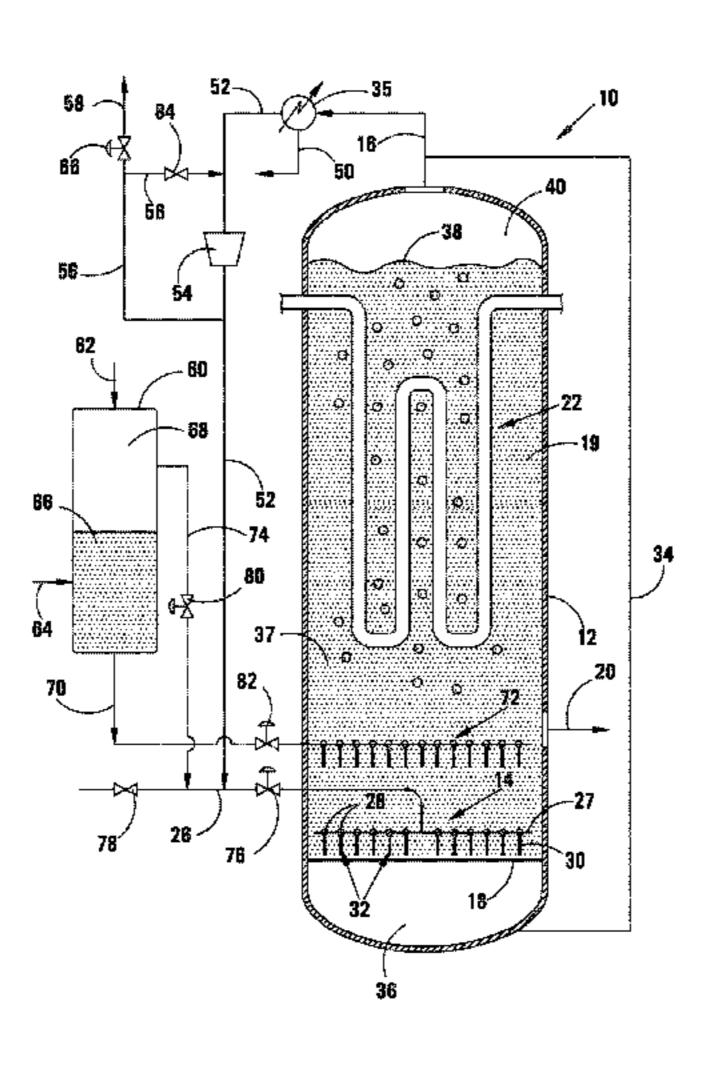
includes abruptly stopping flow of gas from the gas feed line (26) to the gas distribution nozzles (30) to trap gas in the gas distribution nozzles (30) thereby to inhibit slurry ingress upwardly into the gas distribution nozzles (30).
