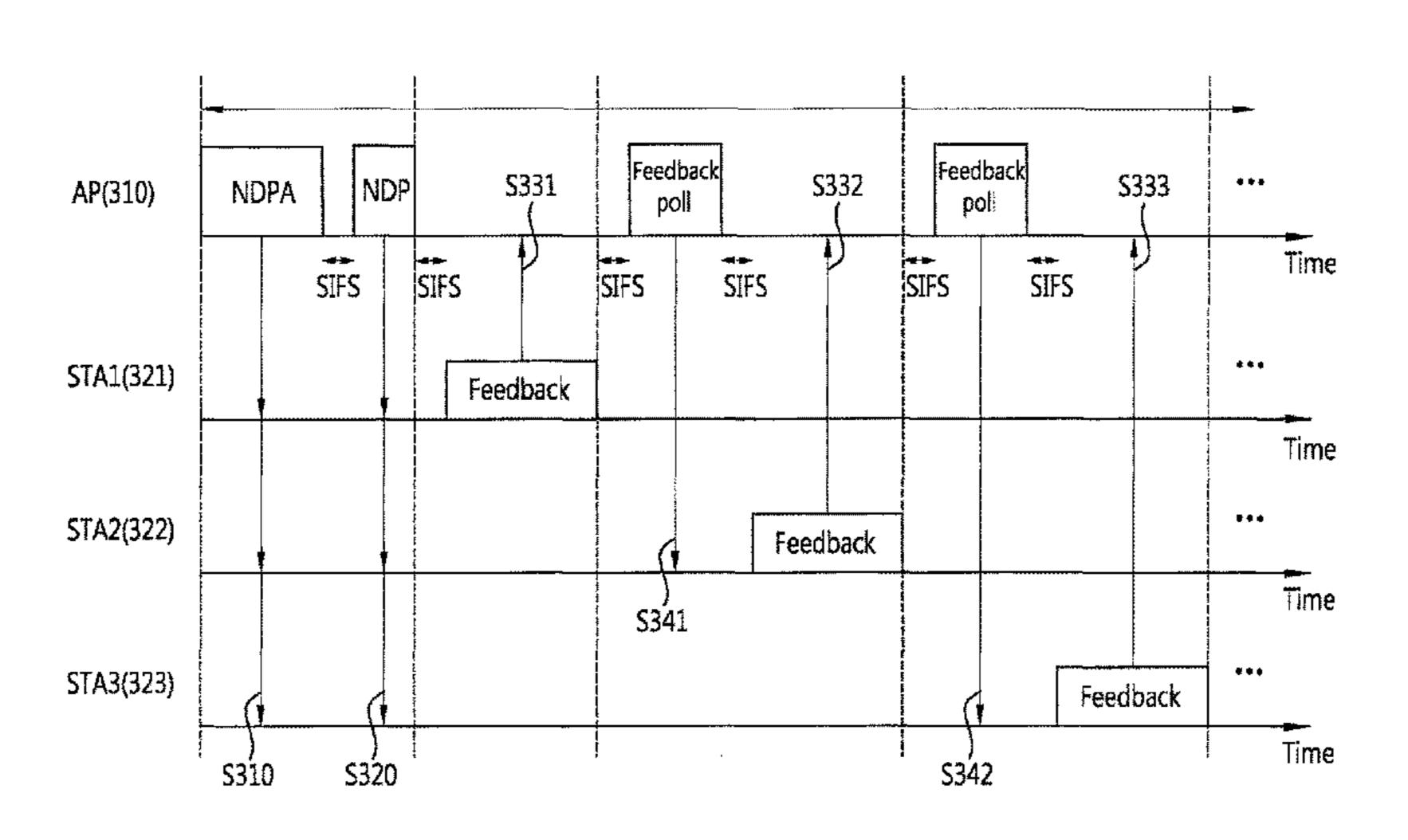
station transmits a second feedback data field including the at least one segment of the first feedback data field to the requesting station.
