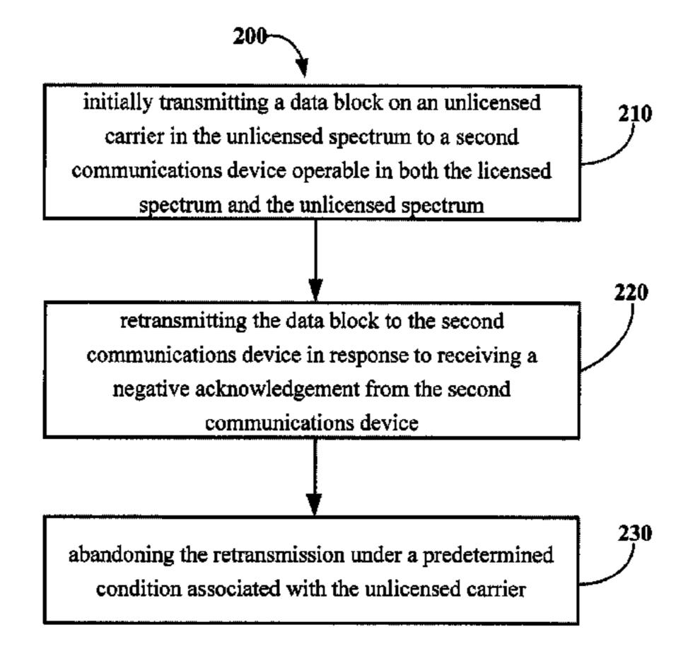
apparatus for data transmission at a communications device operable in both a licensed spectrum and an unlicensed spectrum.
