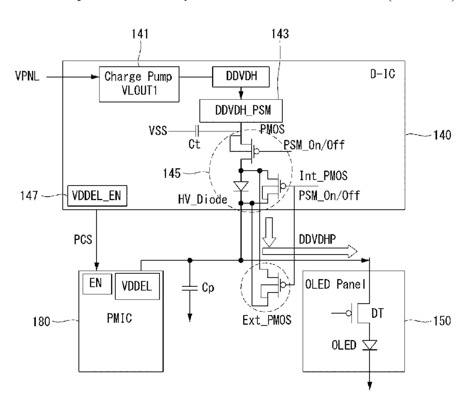
power output from the first transistor, and a second transistor connected to the diode in parallel and configured to output the auxiliary power together with the diode.
