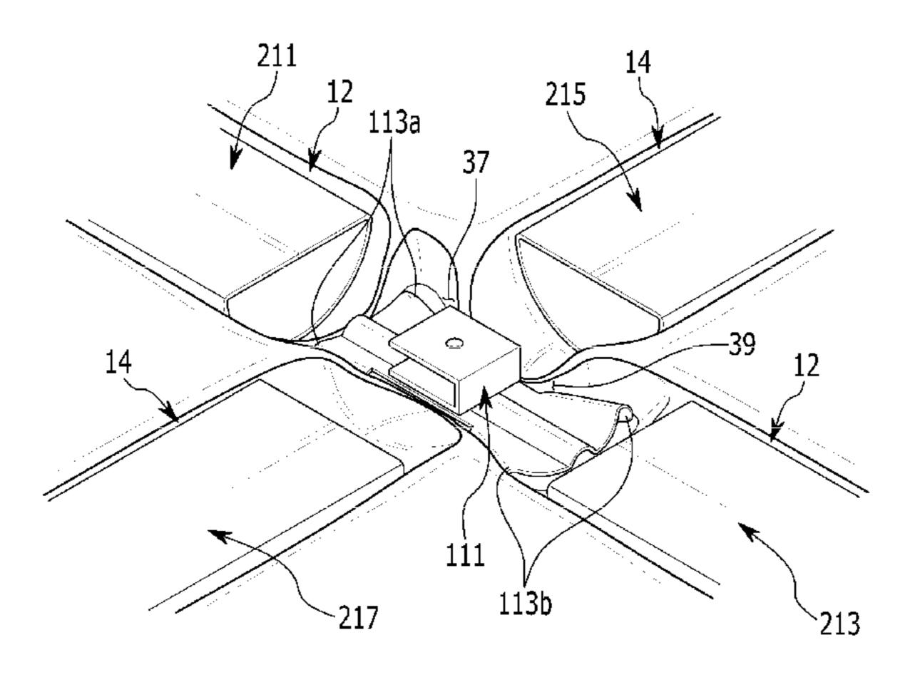
body. The reinforcing member is fixed to inner sides of the first and second corrugated portions by the impact-absorbing plate.
