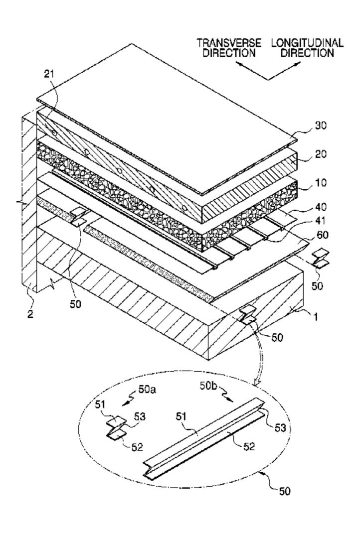
portion of the inter-floor separation layer and an upper plate contacting a portion of the support member to allow the inter-floor separation layer to be spaced apart from the support member.
