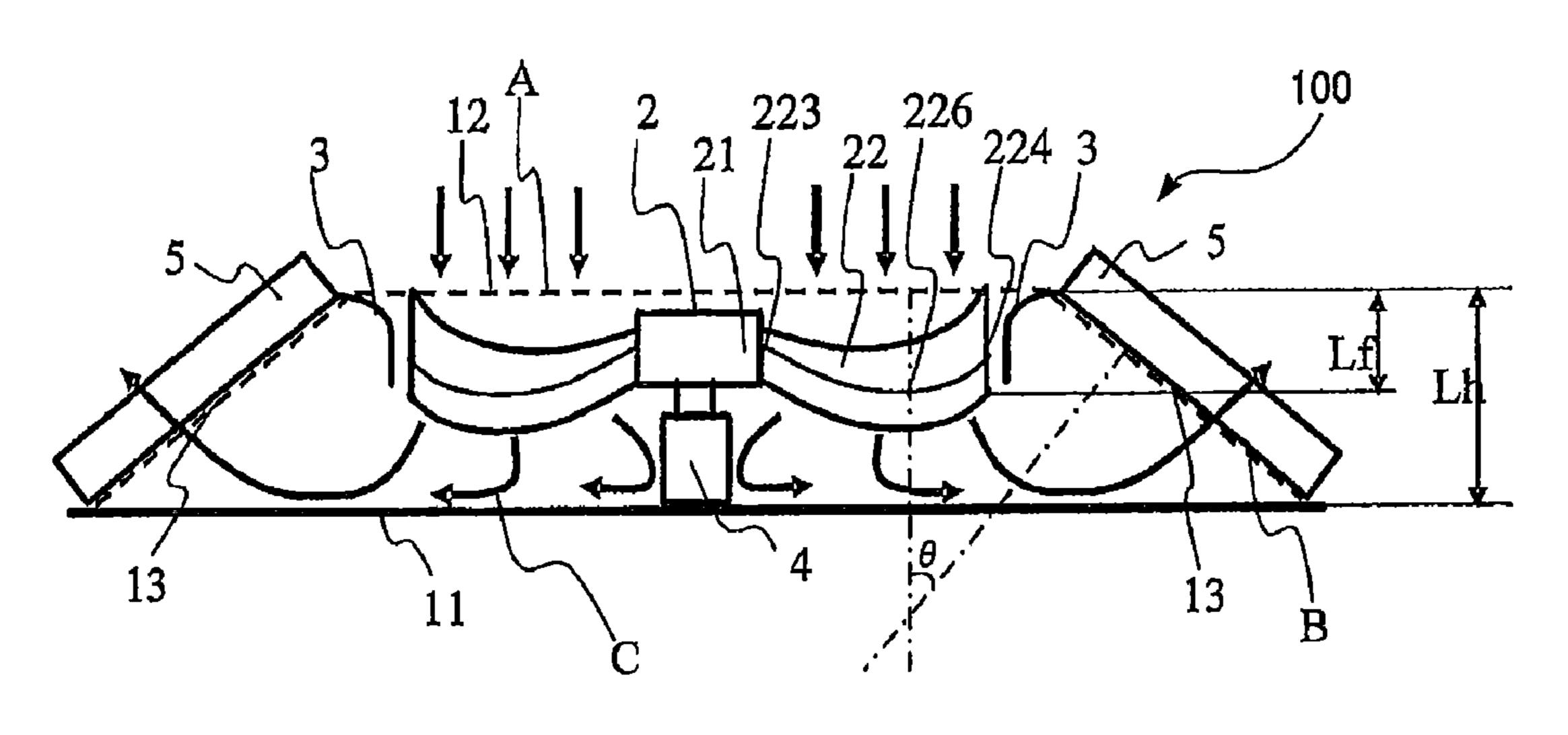
shaft is convexly curved toward the downstream side over the entire area in the radial direction.
