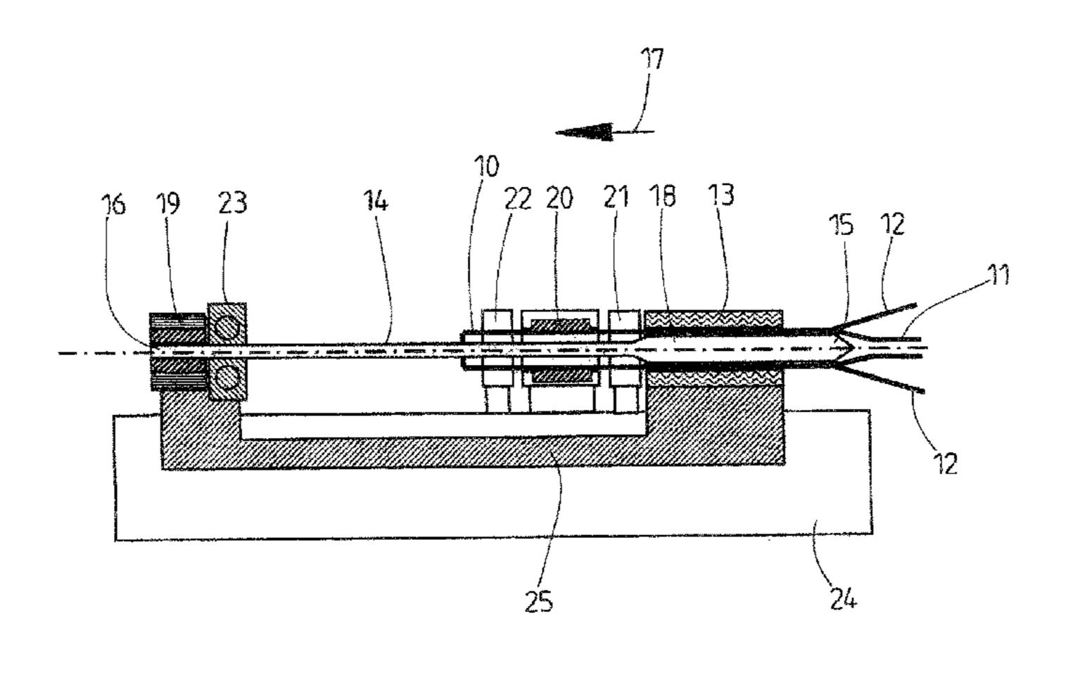
has been formed from a prefabricated reinforcement tube can be pulled over the free front end (15) of the core (14).
