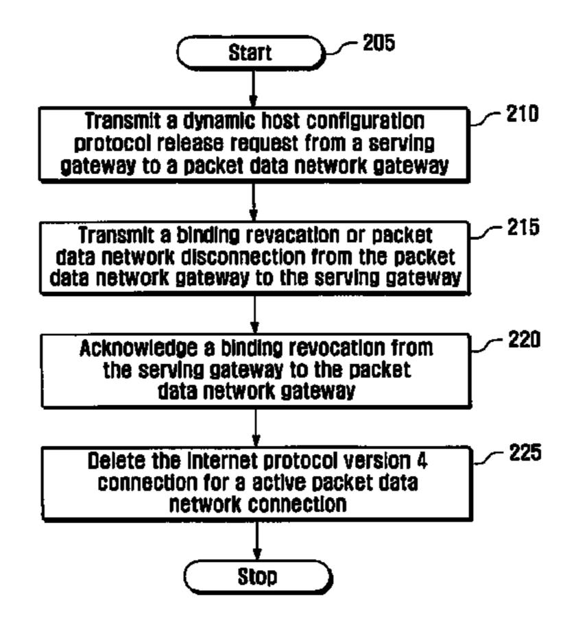
PDN type associated with the PDN connection is an IPv4/v6, which indicates that the UE is allocated both the IPv4 address and the IPv6 address; the PGW transmits, to a Serving GateWay (SGW), a Binding Revocation message including information indicating release of the IPv4 address with the PDN connection remaining if the PDN type is the IPv4/v6; and the PGW receives, from the SGW, a Binding Revocation acknowledge message to acknowledge release of the IPv4 address.
