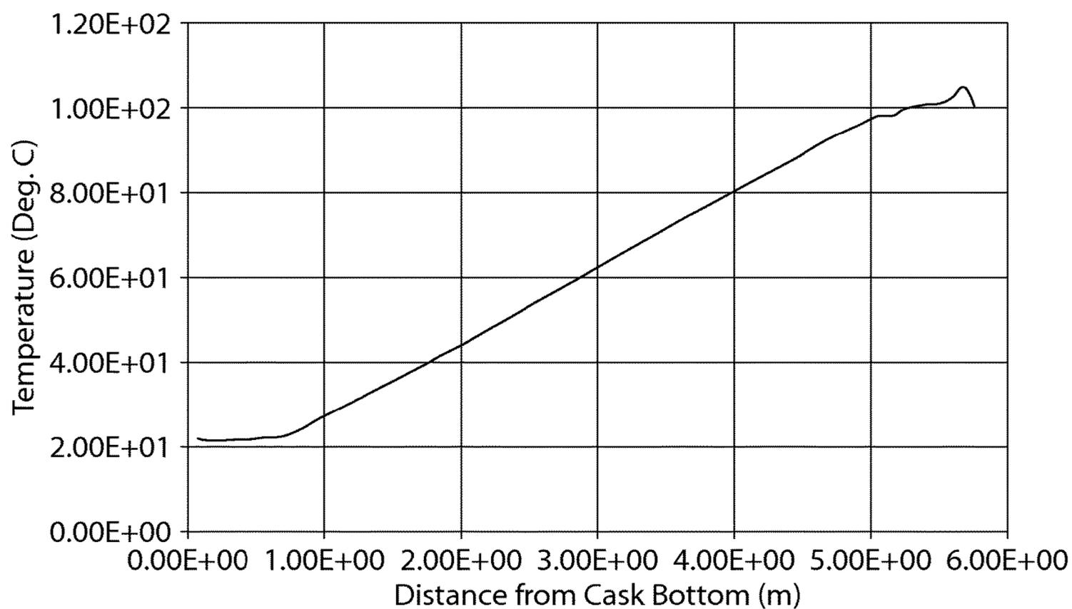
Ventilated Cask Air Temperature Profile Using Prior Art
