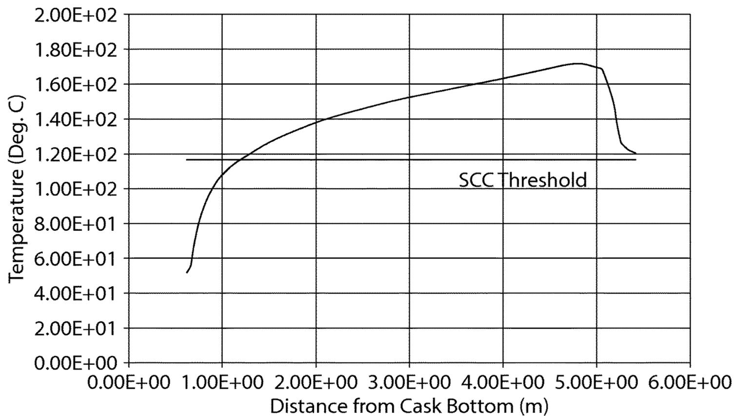
Canister Axial Surface Temperature Profile When Stored
