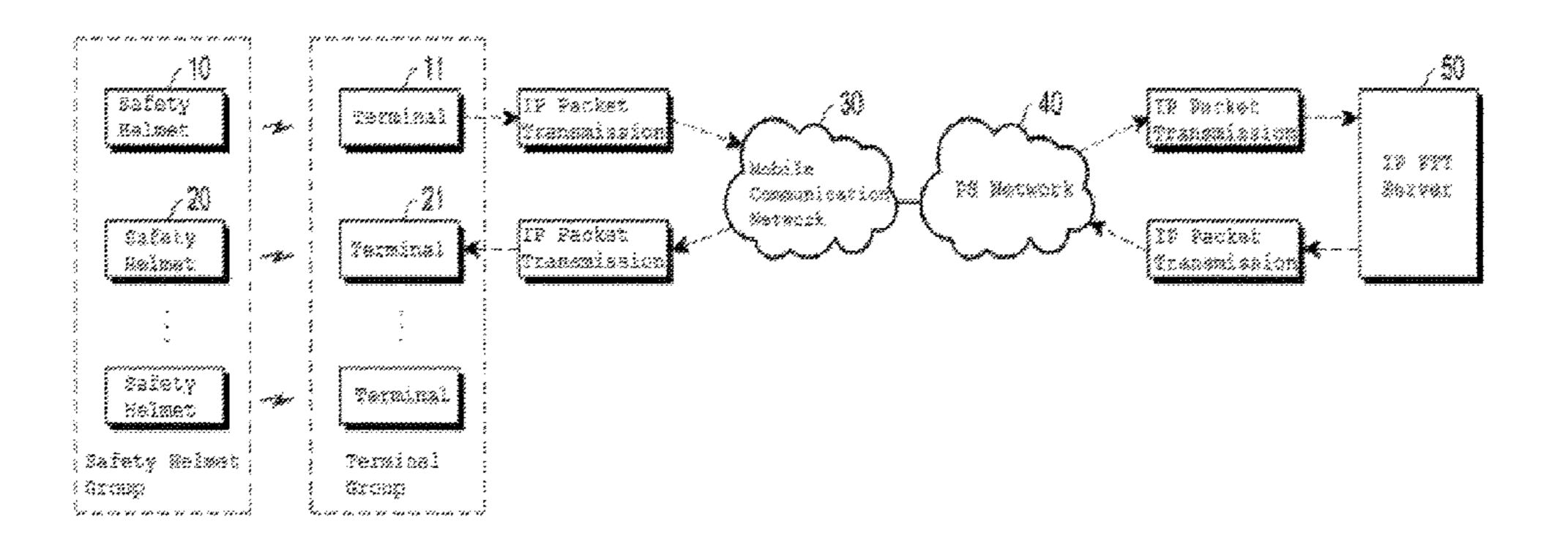
signal or transmitted from the outside; a sound output unit for outputting a voice and a beep sound corresponding to the voice signal and the emergency signal transmitted from the outside; and a control unit for controlling the beep sound so as to be outputted at output time intervals which are set to be different according to the reception strength of the received emergency signal.
