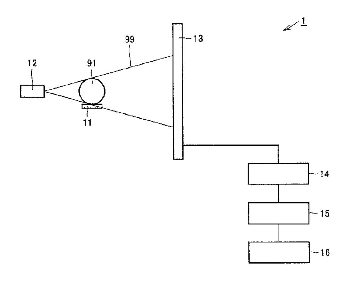
forming an image, data of the X-ray for one circuit around the rolling element is calculated to generate the image.
