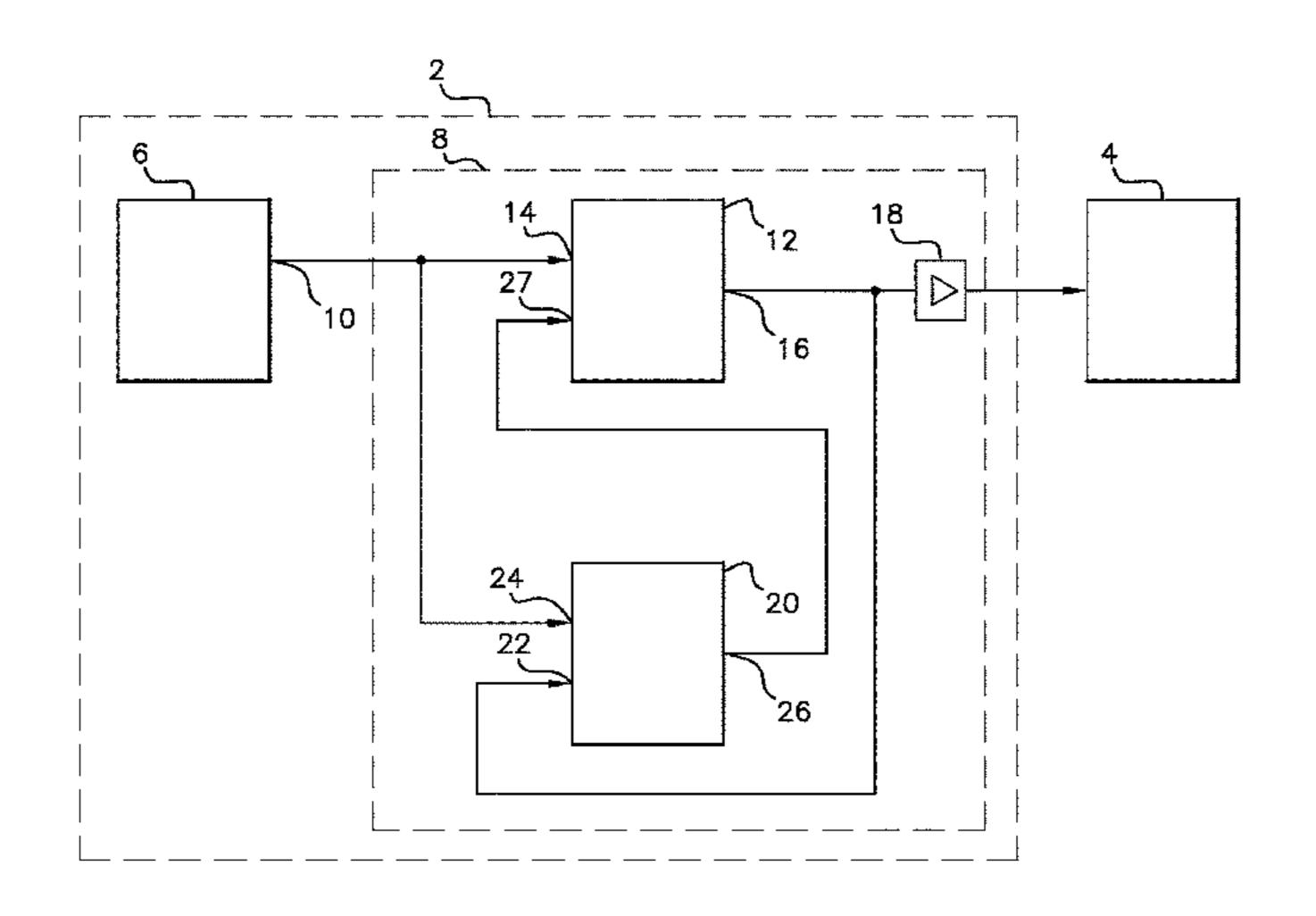
output (16) of the output circuit (8), and control elements associated with time delay elements for interrupting the connection between the output of the output circuit (8) and the component (4).
