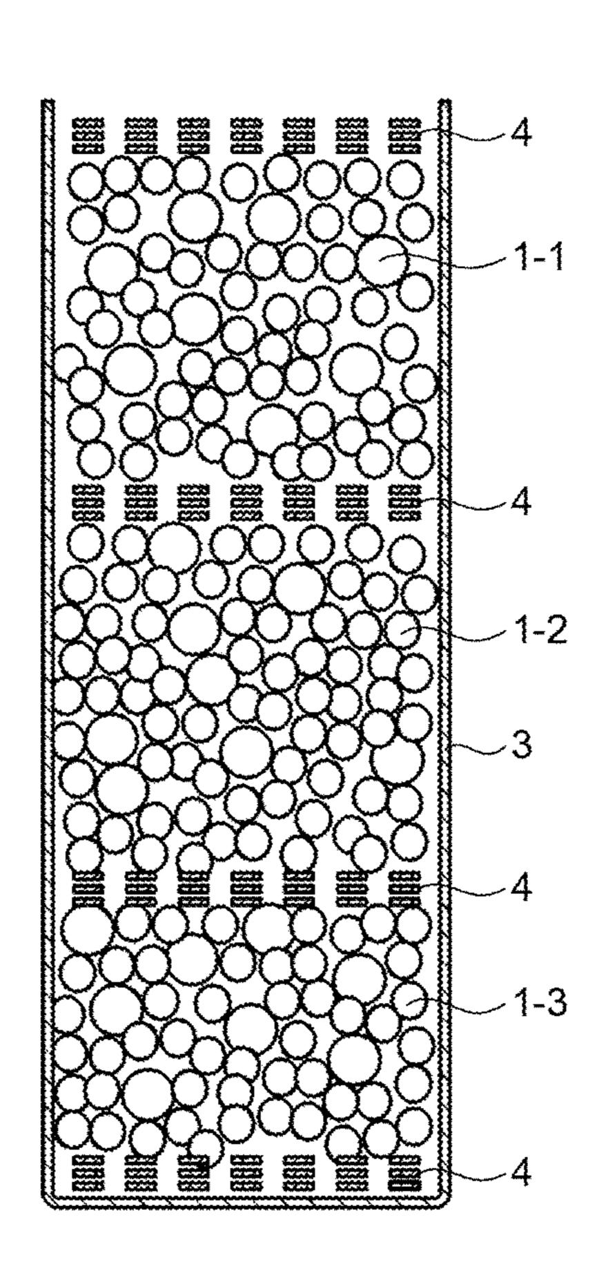
RARE EARTH REGENERATOR MATERIAL PARTICLE, RARE EARTH REGENERATOR MATERIAL PARTICLE GROUP, AND COLD HEAD, SUPERCONDUCTING MAGNET, EXAMINATION APPARATUS, AND CRYOPUMP USING THE SAME
