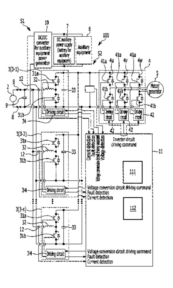
values, wherein the inverter circuit and the boosting circuits perform a regeneration operation of supplying regeneration power to the DC main power supply, peripheral equipment, and/or a DC auxiliary power supply.
