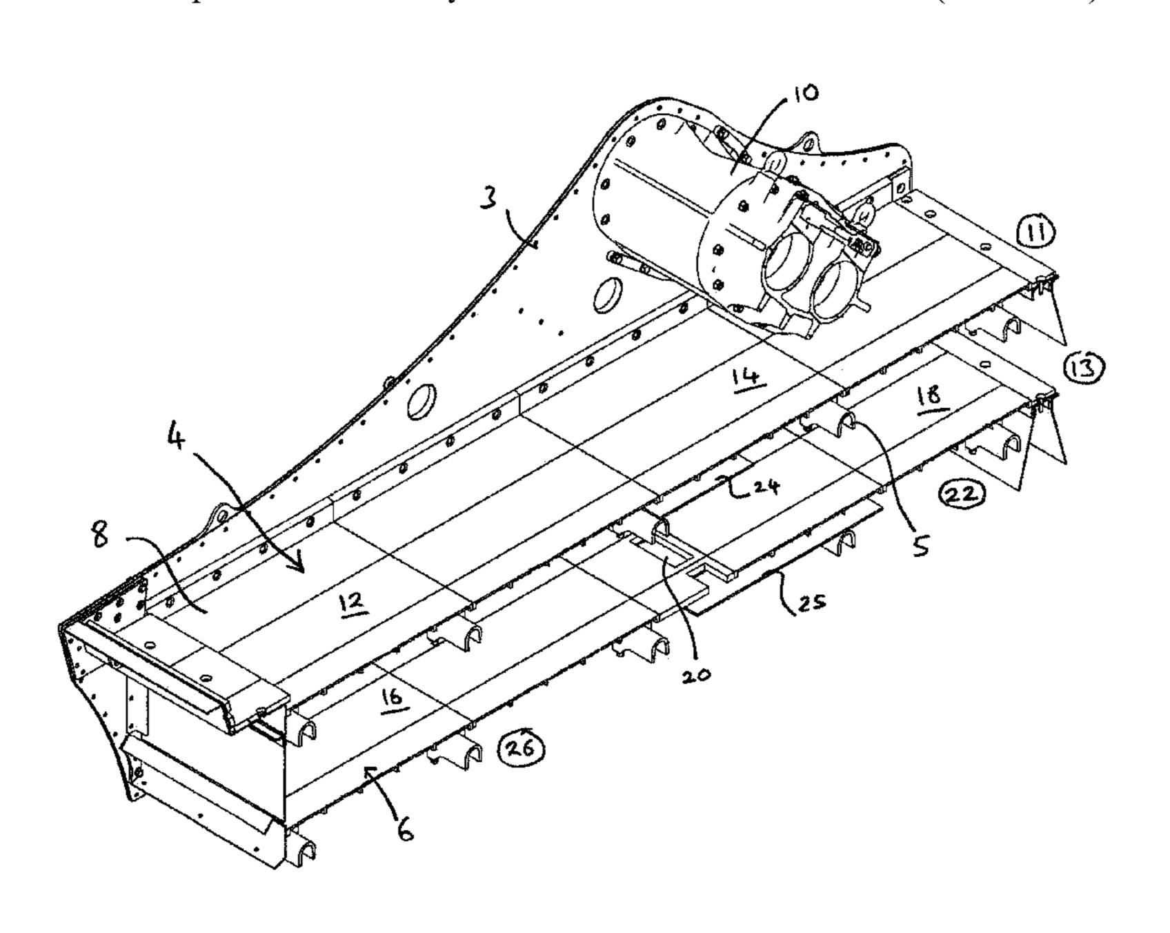
the upper and lower decks and over the gap, whereby material from the upper deck collected on the diverter passes onto the lower deck's second section, thereby preventing undersize material that passes through the upper deck from passing directly through the gap.
