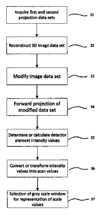
detector; calculating intensity values for a plurality of detector elements from the modified projection data set; transforming the calculated intensity values into scan values; and assigning the scan values to an image matrix.
