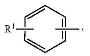
in which R¹ is a C₄-C₁₀ alkyl group; n is an integer of 1-20; m is an integer of 1-3; and X is a counter ion, such as hydrogen, sodium, potassium, lithium, ammonium, or an amine salt such as monoethanolamine, diethanolamine or triethanolamine. In some embodiments, n is an integer of 4 to 10 and m is 1. In some embodiments, R is a C₃-C₁₀ alkyl group. In some embodiments, R is a C₁₂-C₁₄ alkyl group, n is 4, and m is 1.
