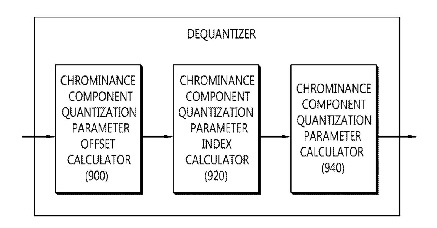
quantization parameter index on the basis of the decoded color difference component quantization parameter offset. Therefore, the present invention enables effective quantization by applying different color difference component quantization parameters according to the size of the transform unit when executing the quantization.
