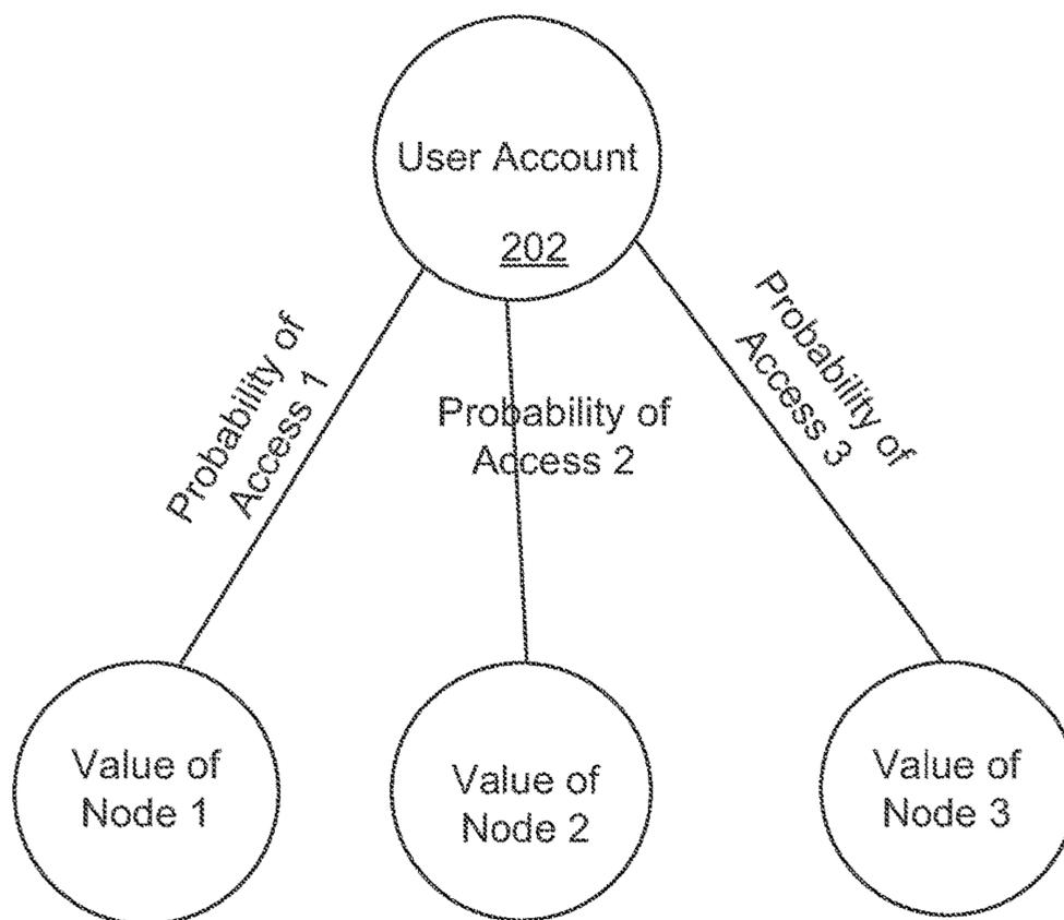
$$\text{Total Expected Value} = (\text{Prob. Of Access 1} * \text{Value of Node 1}) + (\text{Prob. Of Access 2} * \text{value of Node 2}) + (\text{Prob. Of Access 3} * \text{Value of Node 3})$$
