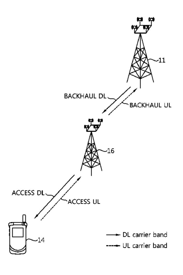
allocation of OFDM symbols in a time domain. Since the radio resource allocation information providing information regarding a time relationship between a control channel transmitted by the BS to a UE and a control channel transmitted by the RS to a UE connected to the RS is provided, the RS can reliably receive a signal transmitted from the BS in a backhaul link between the BS and the RS in a wireless communication system including the RS.
