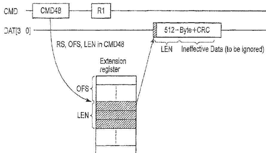
sion register. The extension register records, an information specifying the type of the wireless communication function in a specific page, and an address information indicating a region on the extension register to which the wireless communication function is assigned.
