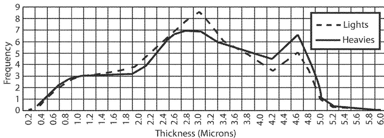
Fiber Wall Thickness Distribution of Fractionated Pulp
