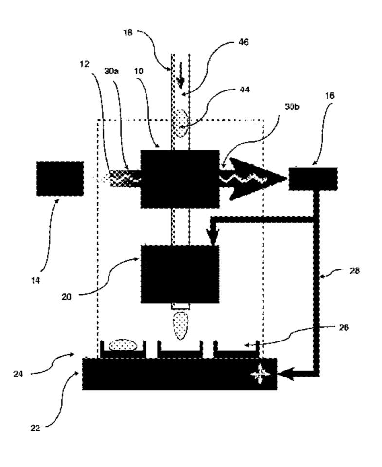
detector and a collector such that the picoliter droplet is isolated by depositing it into one of said wells. The disclosure moreover relates to a method that uses such a system to isolate individual picoliter droplets. In particular the disclosure relates to a method that allows for an analysis and/or further processing of the content of the picoliter droplets that have been isolated from a microfluidic system by depositing them into a well.
