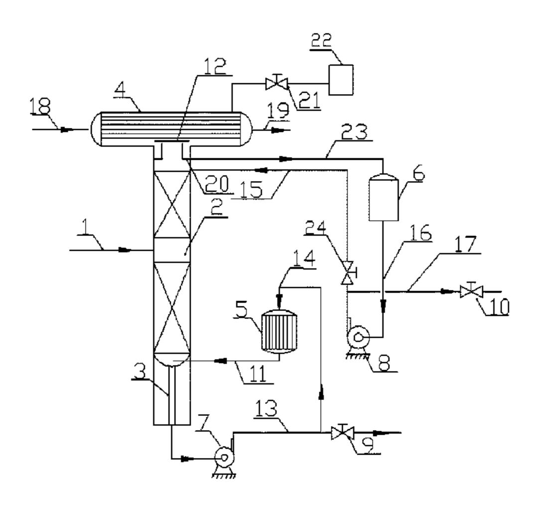
speed circulation system, wherein the tower bottom is an elongated conduit and the falling-film reboiler is in the form of a stout shell-and-tube heat exchanger is provided.
