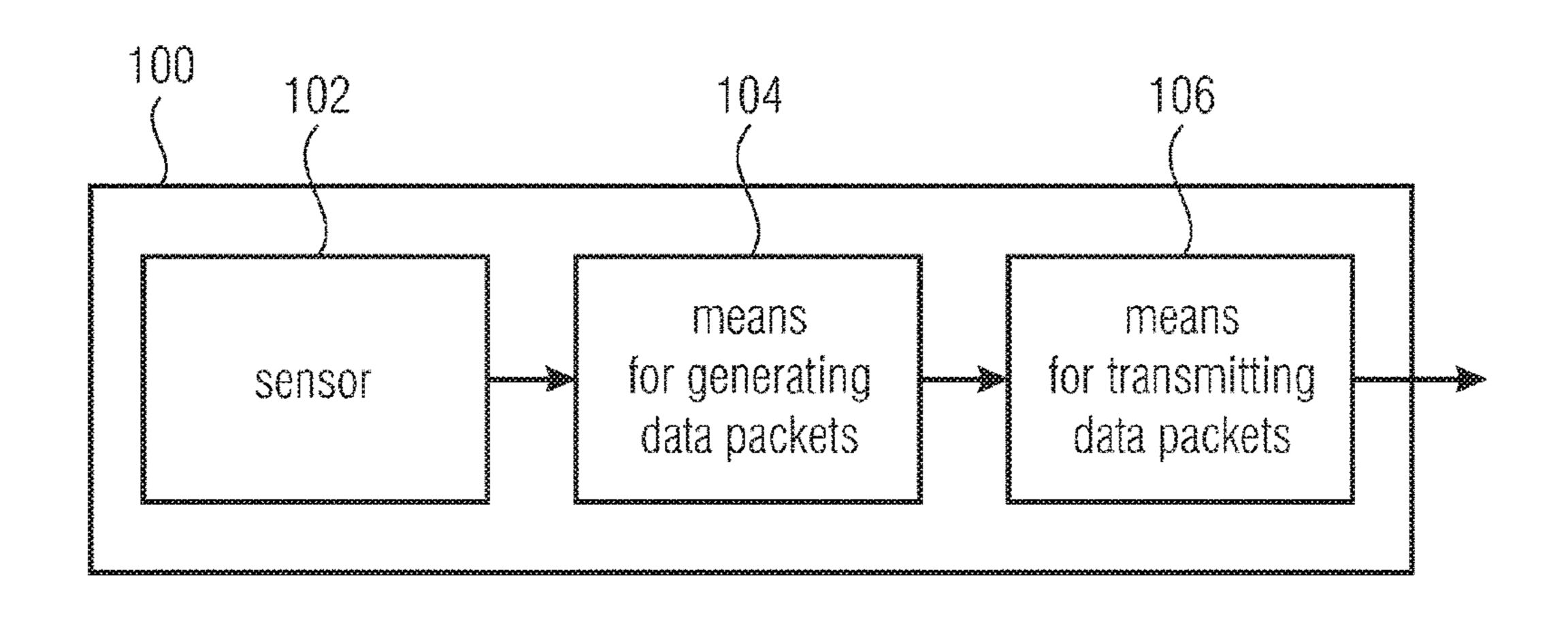
packets, wherein each of the at least two data packets is shorter than the sensor data packet. The means for transmitting data packets is implemented to transmit the data packets with a data rate of less than 50 kbit/s and a time interval via a communication channel.
