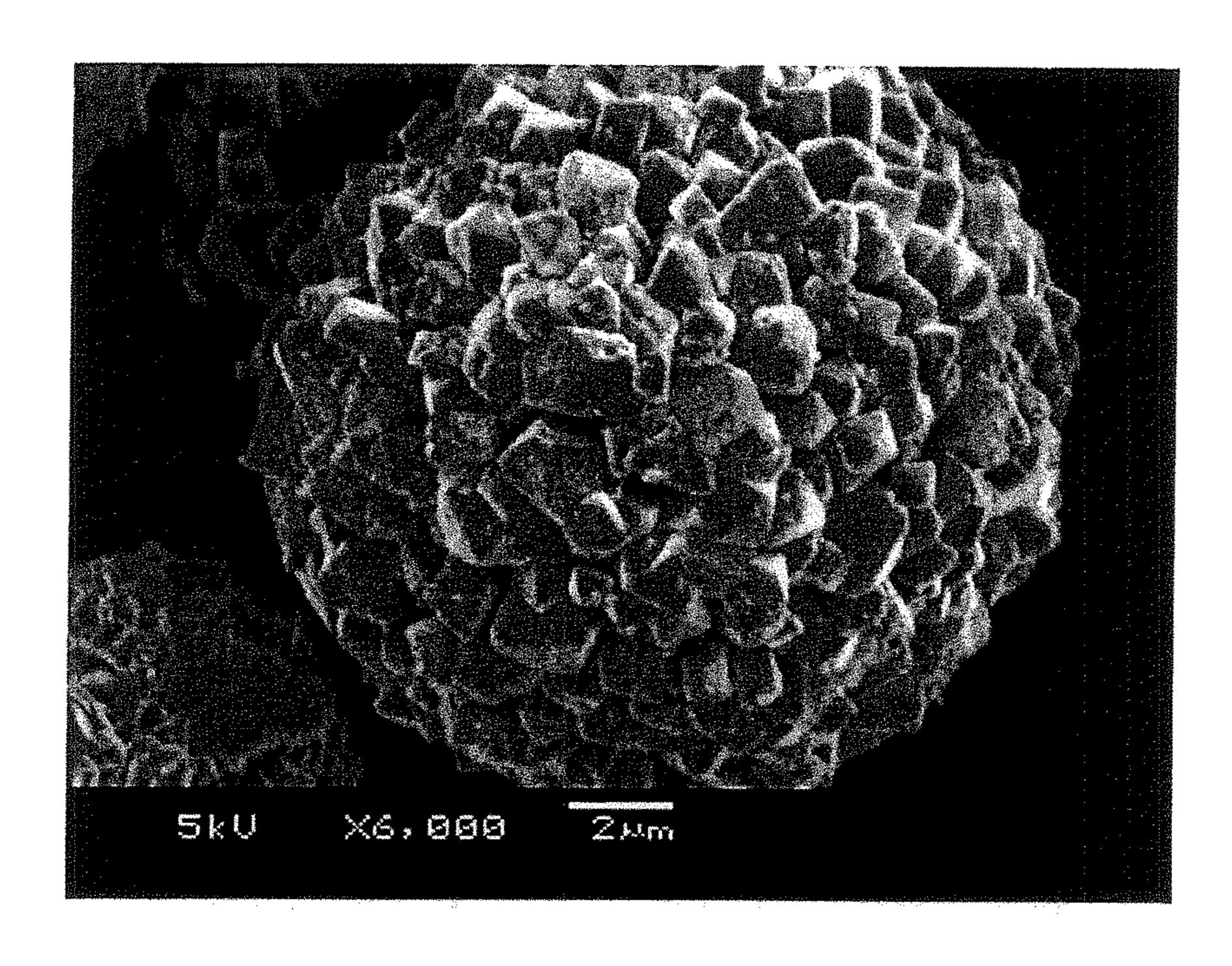
TRANSITION METAL COMPOSITE HYDROXIDE CAPABLE OF SERVING AS PRECURSOR OF POSITIVE ELECTRODE ACTIVE MATERIAL FOR NONAQUEOUS ELECTROLYTE SECONDARY BATTERIES
