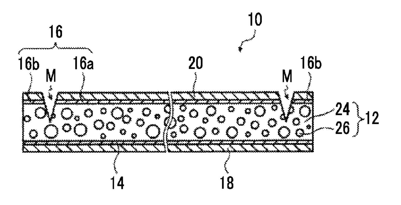
thin film electrode and the protective layer is formed in at least a portion of an outer peripheral portion in a surface direction of at least one of the upper thin film electrode and the upper protective layer, or the lower thin film electrode and the lower protective layer.
