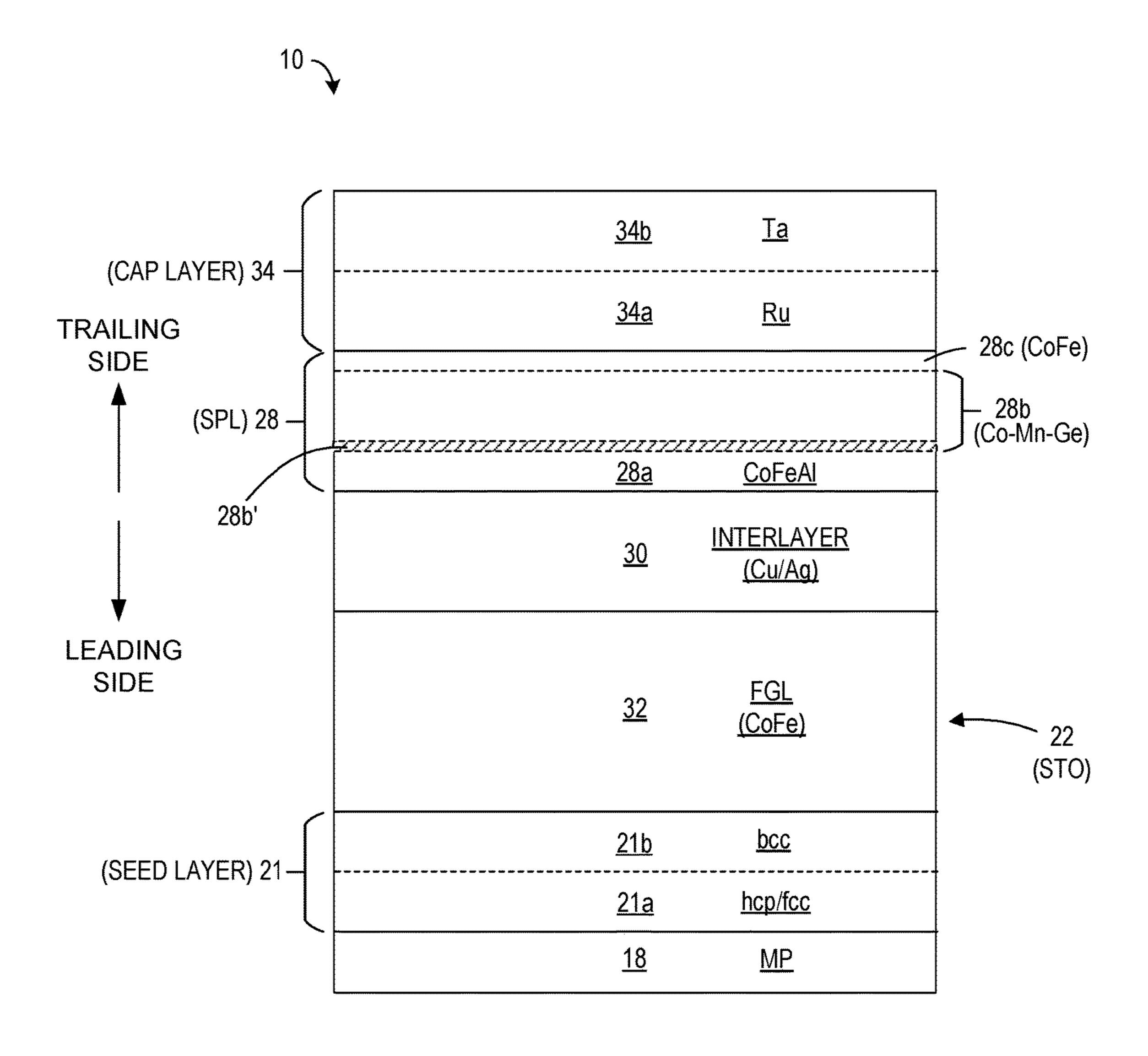
FGL = FIELD GENERATING LAYER SPL = SPIN POLARIZED LAYER STO = SPIN TORQUE OSCILLATOR
