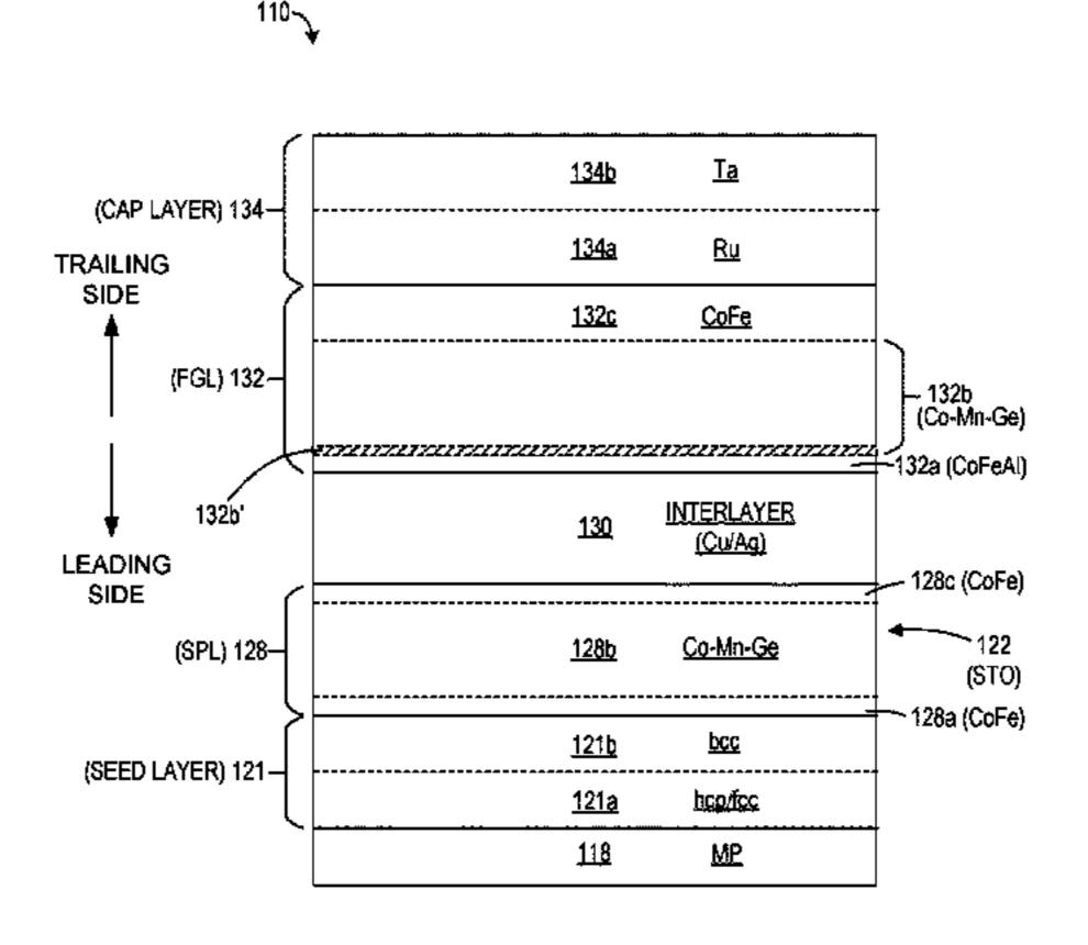
FGL = FIELD GENERATING LAYER SPL = SPIN POLARIZED LAYER STO = SPIN TORQUE OSCILLATOR MP = MAIN POLE
