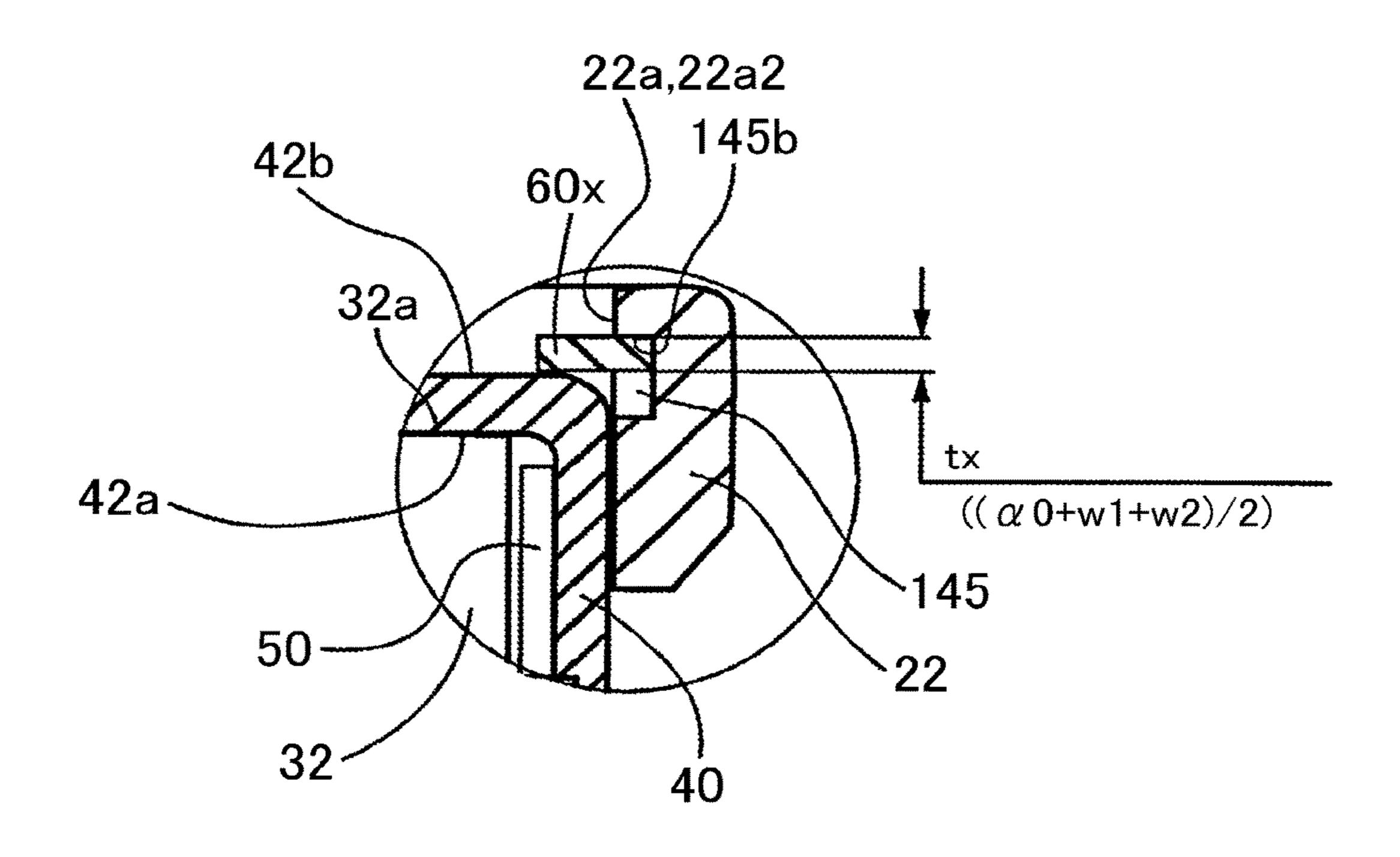
METHOD FOR MEASURING BEARING CUP GAP IN UNIVERSAL JOINT AND METHOD FOR MANUFACTURING UNIVERSAL JOINT TO WHICH THE MEASURING METHOD IS APPLIED
