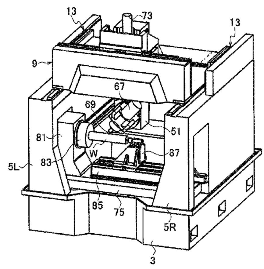
saddle, a lower portion of the up/down slider is provided with a processing head to which a processing tool for processing a work set on the bed is removably and replaceably attached.
