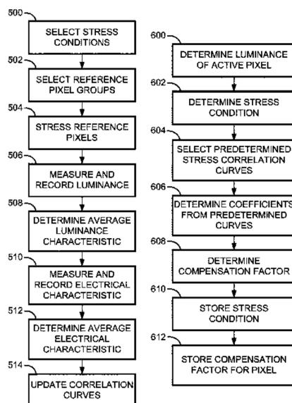
compensation voltage is determined by correlating the stress condition of the active pixel with curves of the predetermined stress conditions.
