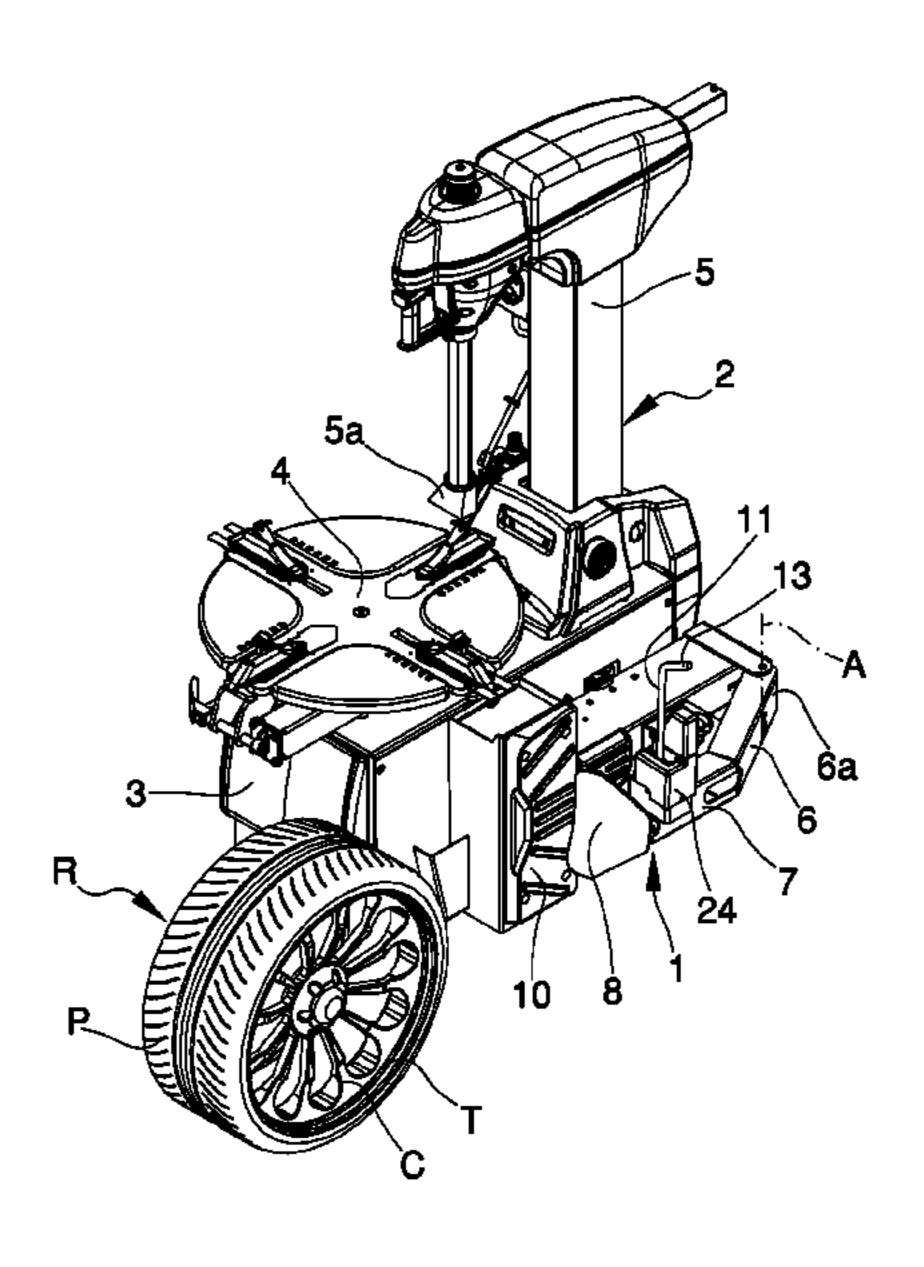
around an oscillation axis substantially horizontal and parallel to the longitudinal direction and is associated with return elements for maintaining the control lever in a substantially vertical balance position, the actuator being controlled in a first direction for bead breaking the tire when the control lever is rotated towards the wheel starting from the balance position.
