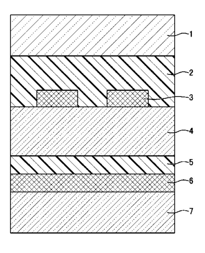
parent inter-layer resin provided between the window and the first transparent film, and a second transparent inter-layer resin provided between the first transparent film and the second transparent film, wherein the first transparent interlayer resin has a dielectric constant greater than that of the second transparent inter-layer resin.
