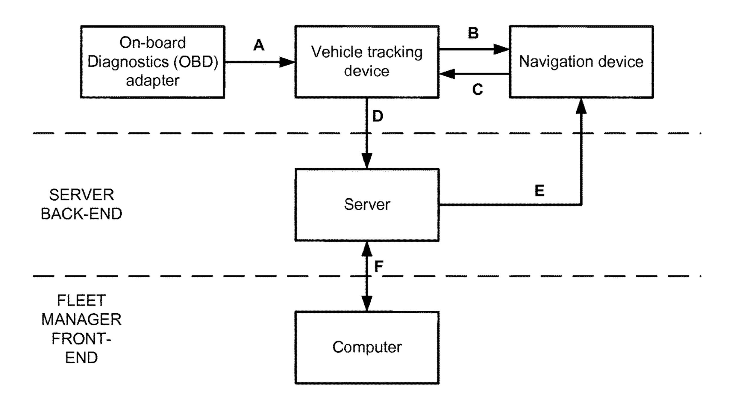
A: current vehicle state data (OBD data and data derived therefrom)
