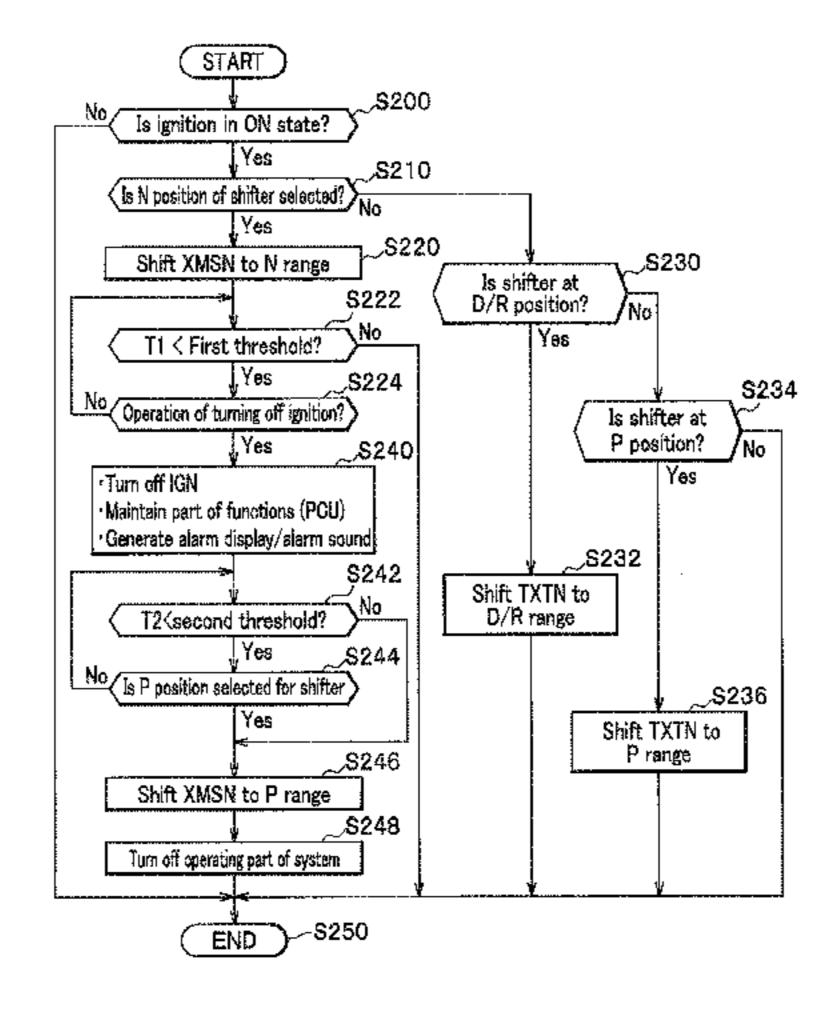
neutral range, when the vehicle power source turns off or when the drive power source stops, until the elapse of a first prescribed time after the shift selection unit receives a neutral position selection while the vehicle power source is on or while the drive power source is driving.
