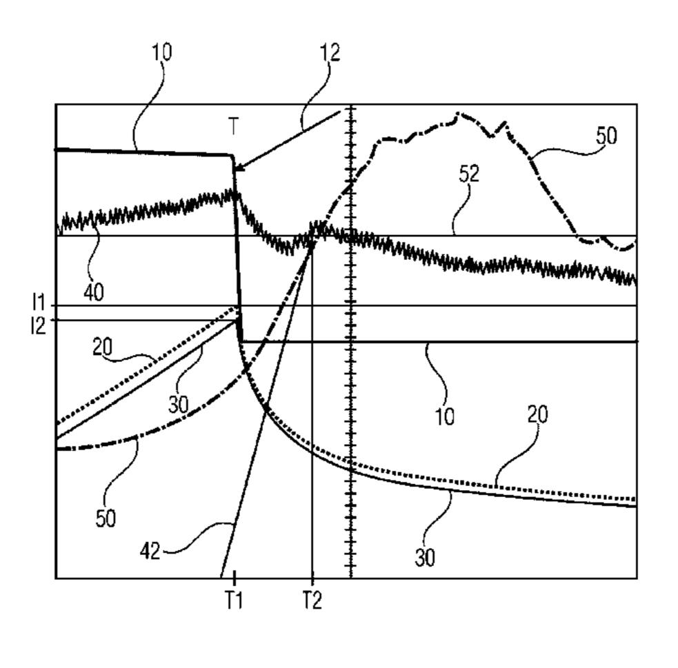
progressions of the current intensity, and determining a point in time at which the differential progression exhibits an extremum, which corresponds with the point in time of the predetermined open state.
