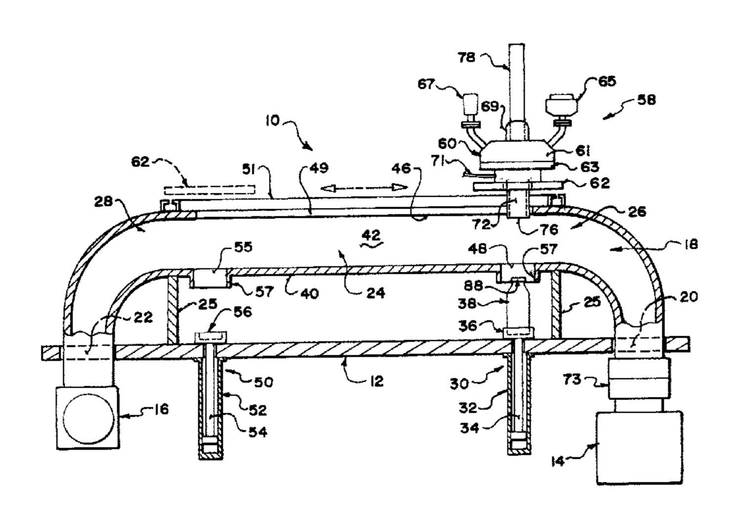
and means for removing the dehydrated material from the waveguide. In the method of the invention, the container of biological material is put in a microwave waveguide open to the atmosphere, a vacuum is applied to the container, the material is frozen and is radiated to dehydrate it. The dehydrated material is then removed from the waveguide.
