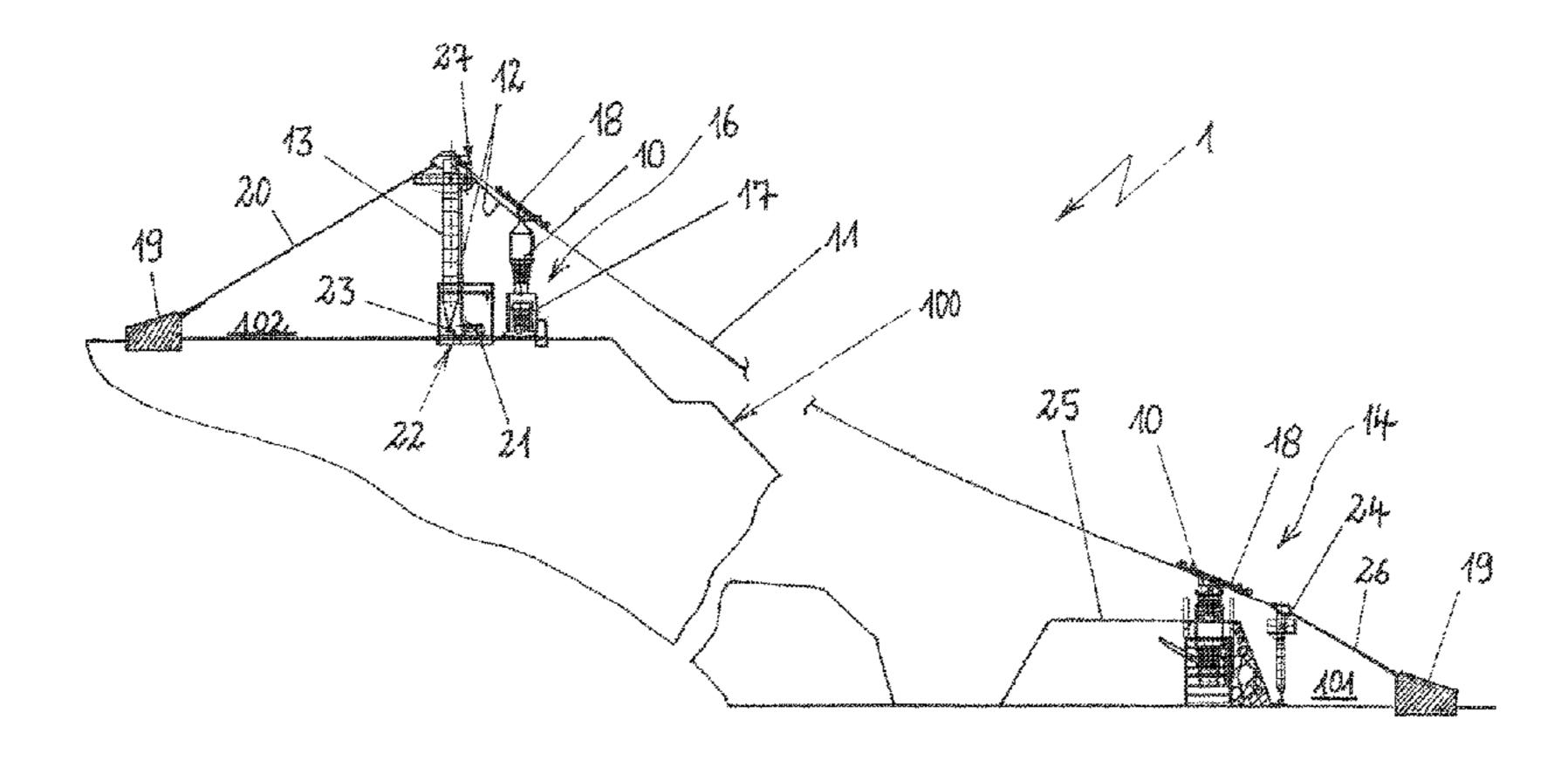
one bearing cable for load-bearing and control and one traction cable for moving the conveying container may be provided. At least at the upper height level, a support element may be disposed, to which the bearing cable is attached and on which the traction cable is guided.
